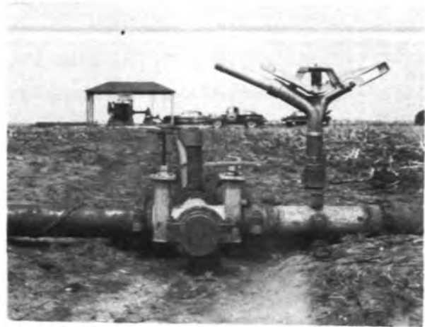
FIGURE 14. THIS NOZZLE SPRAYS 750 GALLONS-PER-MINUTE ON CORN FIELD NEAR EL PASO, ILLINOIS.
